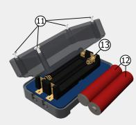
Unscrew the bolts 1 at the back of the sensor module and place the included AAA batteries 2 into the battery holder 3.
