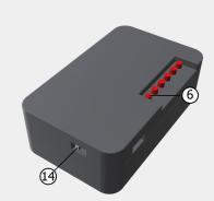
Turn the power switch <sup>(1)</sup>/<sub>(1)</sub> to the right to change to battery power mode, and then press and hold the power button <sup>(6)</sup>/<sub>(6)</sub> for about 2 seconds. if you a plug headphone to the module you will hear two-tone alert sounds indicating that the device is turned on.
