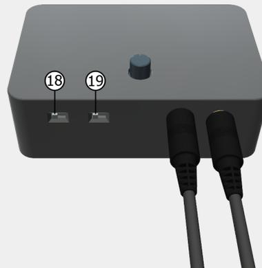
Turn on the sensor module by sliding the power switch to the right ⑱.
